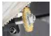
Powered chip removal brush
