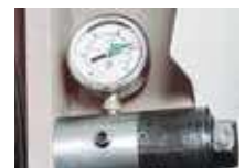
Blade tension display For monitoring the optimum saw blade tension even while the machine is in operation (standard)
